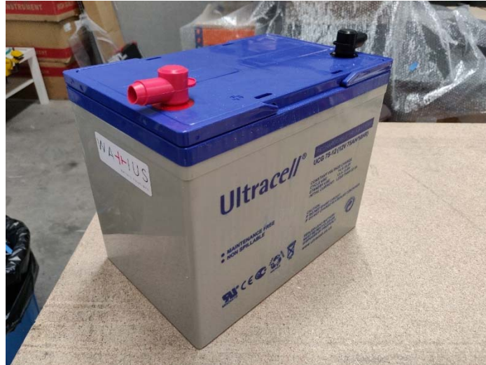
Figure 17. Ultracell UCG75-12 valve regulated lead-acid battery.
